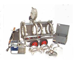
The clamps are designed for side loading of pipe, which facilitates the removal of the machine from a completed pipe joint and especially from trench work. Pipe alignment is simply achieved by adjusting the unique eccentric cam mechanisms attached to the fixed clamps.
