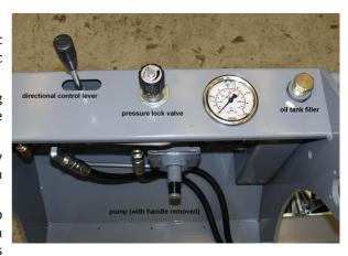
available to isolate the pump from the carriage cylinders and pressure gauge. However, it is only safe to close the lock valve after the weld zone temperature has cooled enough so that the rate of plastic shrinkage and pressure loss is slow.
