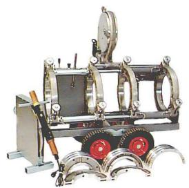
The clamps are designed for side loading of pipe, which facilitates the removal of the machine from a completed pipe joint and especially from trench work. Pipe alignment is simply achieved by adjusting the unique eccentric cam mechanisms attached to the fixed clamps.
